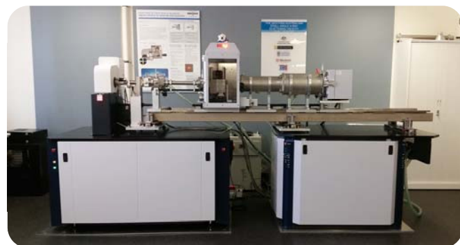
Bruker NanoStar small angle X-ray scattering instrument.
